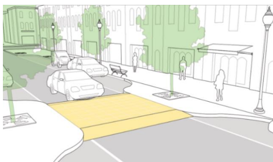
Safe pedestrian crossing on a speed table (ITDP)
