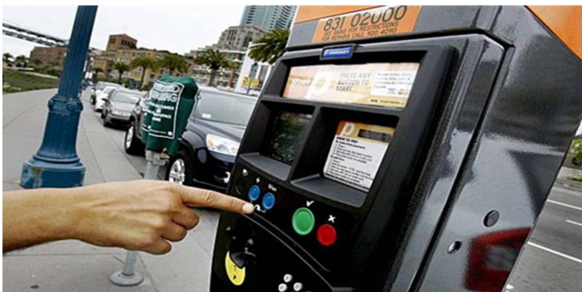
Figure 39. Multi-space parking meters which accept credit cards and coins, San Francisco, USA Photo: Brant Ward, The Chronicle
