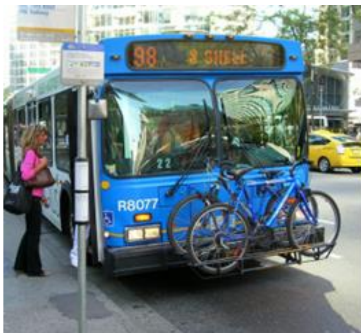
Figure 41. Bike fastening in front of the bus, Vancouver (Canada), 2015 Photo: Stephen Rees
