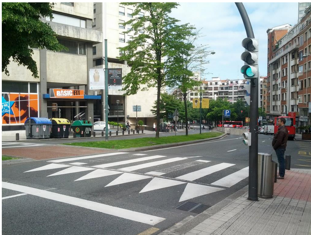
Figure 54. Raised crosswalk with “sharks' teeth” and median refuge, Bilbao, Spain (2015) Photo: Eric Fischer
