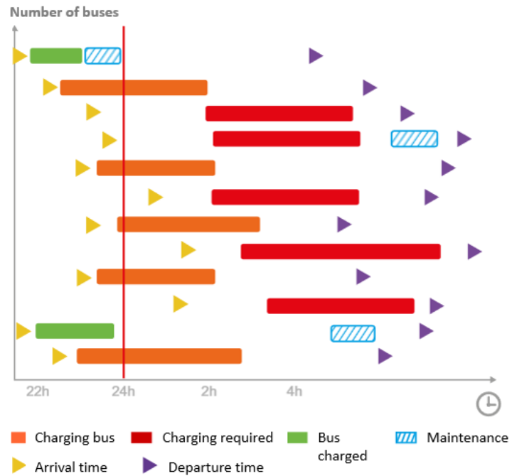
Figure 82. Example of recharge management system (source: C-Way)
