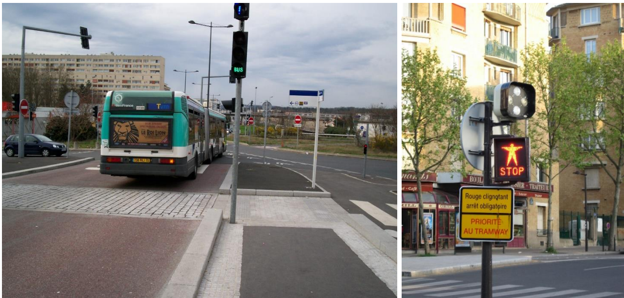
Figure 105. Traffic light priority system in Paris, France - left: bus priority signal / right: pedestrian no-crossing signal (source: Wikimedia Commons)
