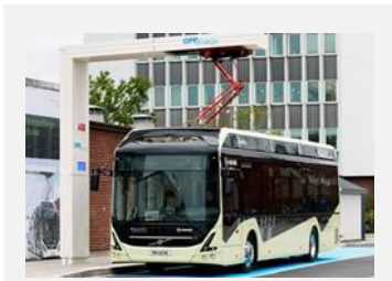
Inverted pantograph (source: ABB)
