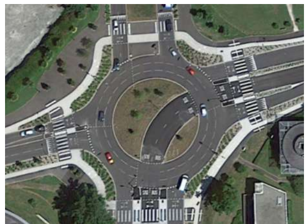
Example of crossroads crossing treatment for BRT with a compression – Pau (France)
