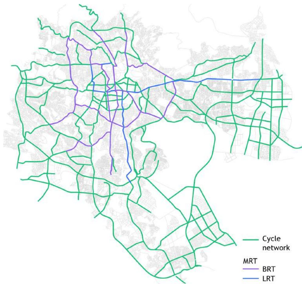
Figure 16. Cycle tracks are needed along streets with heavy vehicle traffic. Implementation will prioritise streets with large cycle volumes, streets near bicycle sharing stations, and streets along rapid transit corridors.
