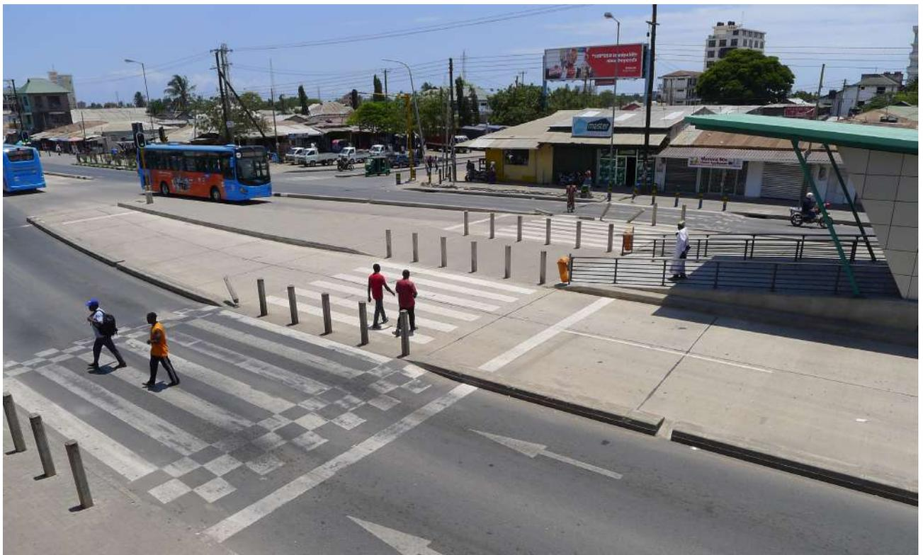
Figure 18. Safe at-grade pedestrian crossings, such as this speed table crossing in Dar es Salaam, provide easy, convenient access to rapid transit stations.
