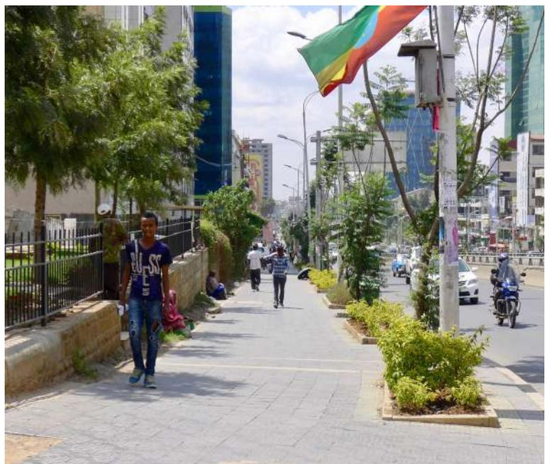
Figure 9. Well-design footpaths have three main zones: the frontage zone, pedestrian zone, and the furniture zone. The width of the pedestrian zone is context-specific and should be at least 2 m.
