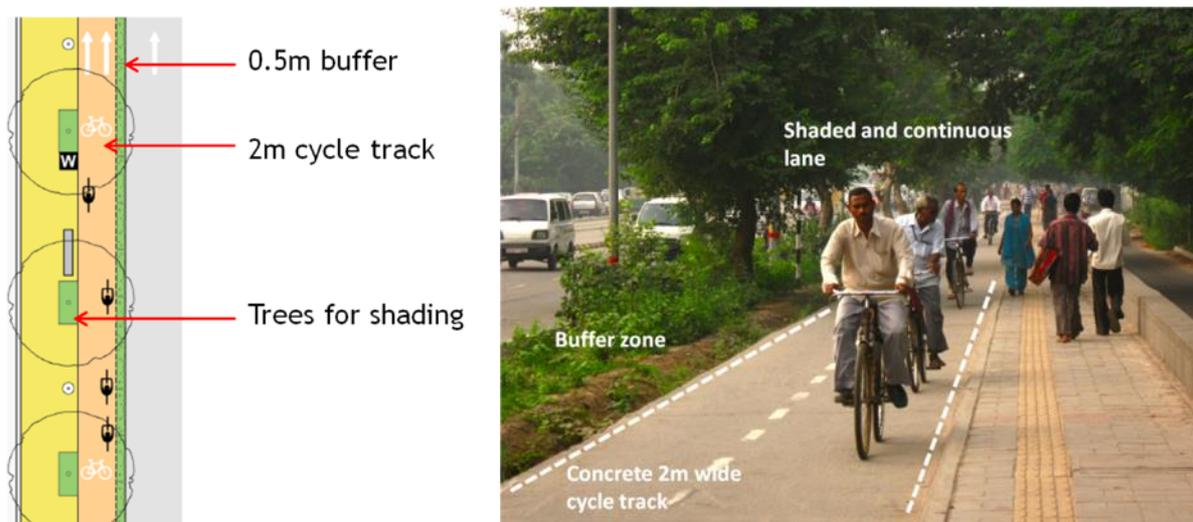
Figure 66: Cycle tracks should have a minimum width of 2 m and an elevation of 100-150 mm above the carriageway. Trees along the cycle track provide shade and comfort for cyclists.
