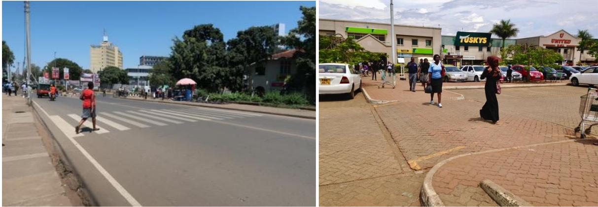
Figure 16: The lack of traffic calming and universal access hinder safety at crossing points (left). A traffic-calmed and accessible crossing is present at United Mall (right).
