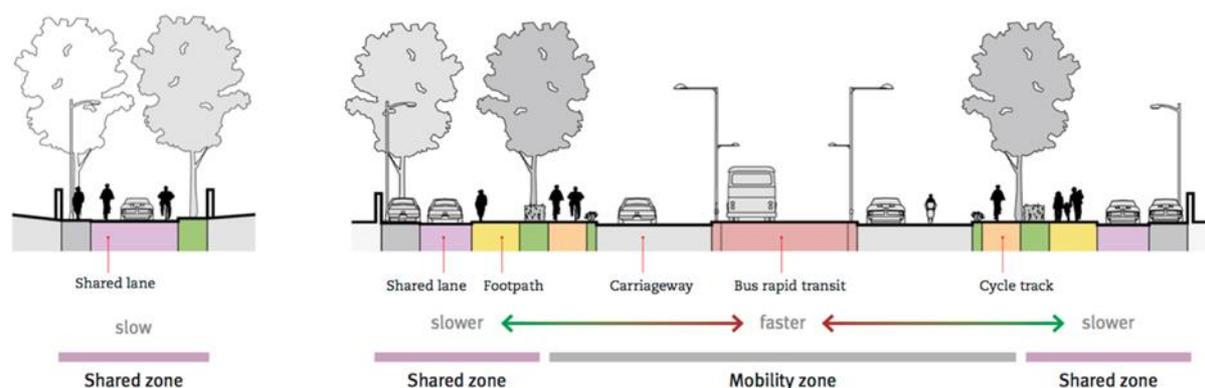
Figure 62: Smaller streets can function as shared spaces where pedestrians walk together with slow-moving vehicles (left). On larger streets with heavy vehicles and faster speeds, separate space for pedestrians and cycles is needed (right).
