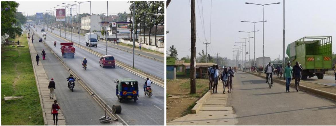
**Figure 15: Wide shared lanes for pedestrians and cyclists along Nairobi-Busia highway. The NMT facilities are often encroached by motor vehicles, introducing safety risks for pedestrians.**
