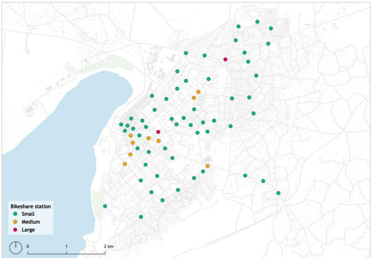
Figure 74: Proposed station locations for a first-phase bikeshare system. Small stations should have 10 docks, medium stations with 20 docks and the large stations with 30 docks.
