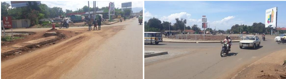
Figure 57: Wide turning radii at intersections encourage drivers to move at high speeds, thus endangering NMT users.
