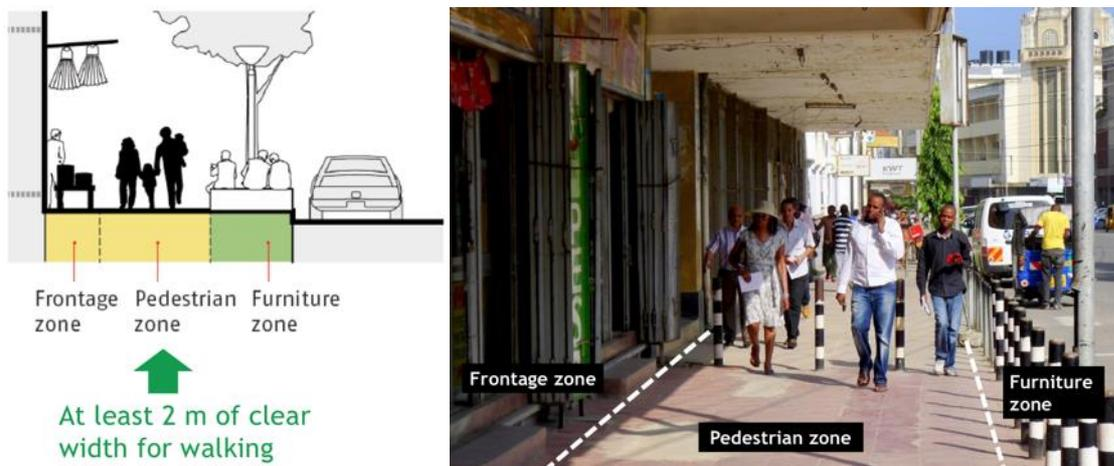
Figure 63: A well-designed footpath has three main zones: the frontage zone; pedestrian zone, with a minimum clear width of 2 m; and the furniture zone.
