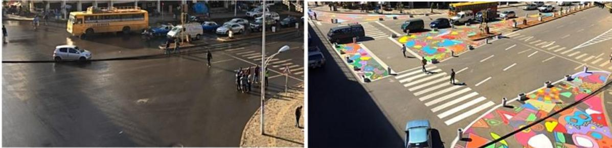
Figure 68. Before and after images of intersection modifications in Addis Ababa to reduce lane widths and turning radii for motor vehicles in order to improve pedestrian safety.
