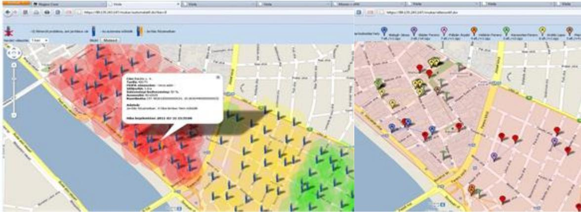
Figure 82. Budapest’s parking management system provides real-time information on the status of parking fee collection (left) and enforcement personnel (right).
