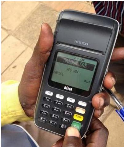
Figure 50: Handheld device used to monitor parking fee payment.
