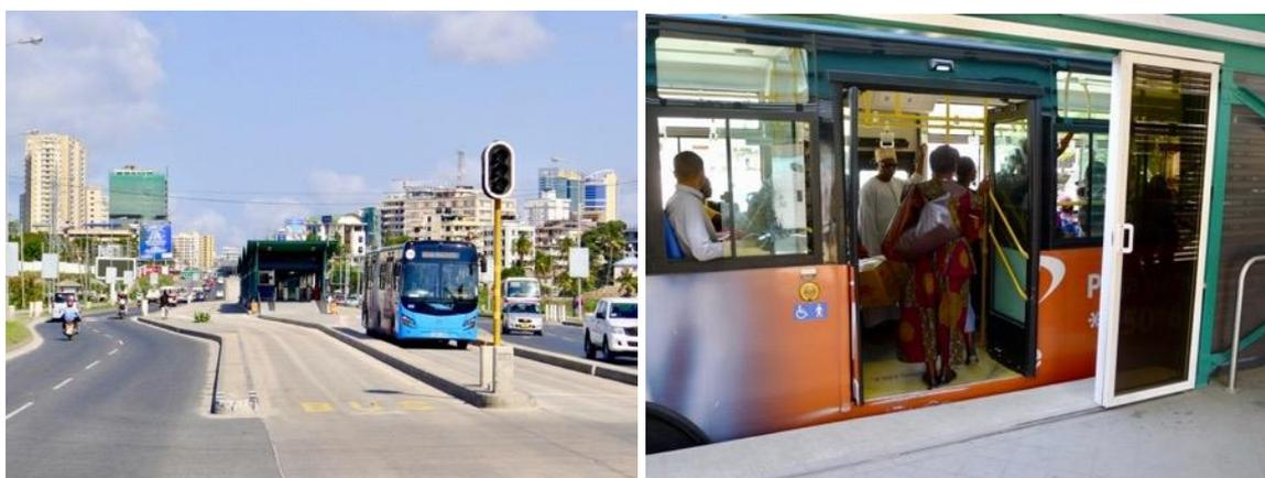
Figure 80. BRT systems, such as the Dar es Salaam BRT system pictured here, incorporate features such as dedicated median bus lanes and level boarding from central stations.
