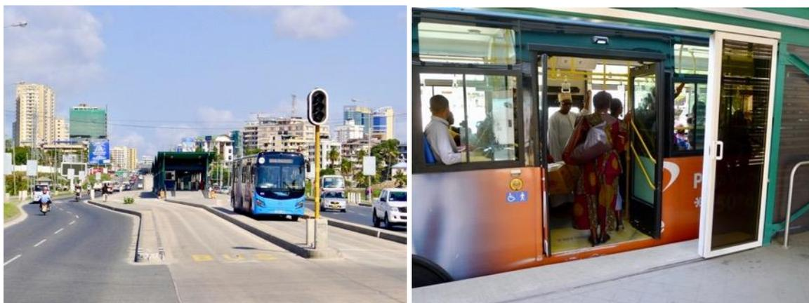
Figure 80. BRT systems, such as the Dar es Salaam BRT system pictured here, incorporate features such as dedicated median bus lanes and level boarding from central stations.
