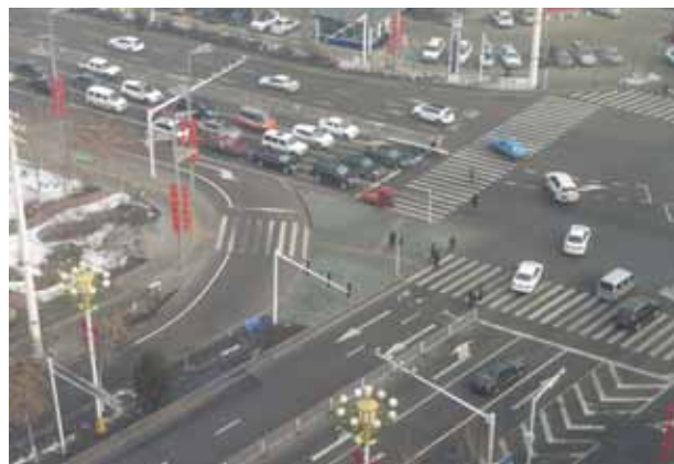
Signalized intersections. Signalized intersections across the CAREC road network vary greatly in the level of safety and amenity provided to pedestrians. Too many have insufficient clearance times, leaving some pedestrians caught in traffic (photo credit [left photo], Ministry of Transport, Tajikistan).
